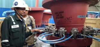
OSL's Stud Tensioning service is an accurate method of tightening threaded fasteners and subsequently inducing load through advanced hydraulic technology – all without directly turning the nut thereby avoiding frictional losses. Stud Tensioning insures that gaskets are compressed as required by the manufacturer in order to achieve optimum joint integrity.
