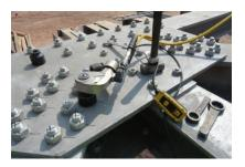
This service provides a simple and safe method for ensuring controlled tightening and loosening of bolts. A wide range of light, compact, safe and easy-to-use hydraulic, pneumatic, and electric torque tools are available.
